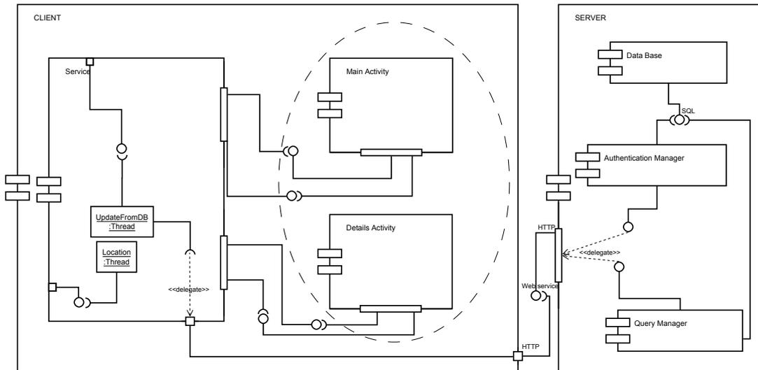
Figure 2.2: The components diagram of the client-server architecture, in the UML standard. The client side is designed as a mobile application for the Android operating system; the server side provides contents to mobile clients through a web service.
