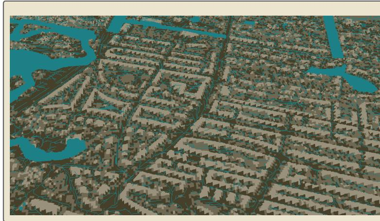
Figure 3.8: 3D representation of DEM and overland flow paths in Rotterdam.
