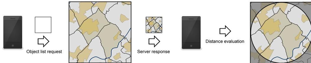
Figure 2.5: The logic behind an object list remote query: a squared bounding box on the Android client is computed, then the database server performs a simple range query on that box. Finally the Android client is responsible of tasks like object sorting and real distance evaluation.
