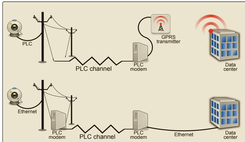
Figure 3.2: A representation of the physical channel used for communication, exemplified by two possible configurations. The main idea comes linking the WTC to the city kernel over the urban power supply.
