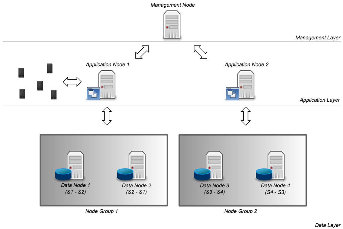
Figure 2.4: The provider side infrastructure in a distributed context. Data base logic is horizontally partitioned in shares (here S1, S2, S3, S4). Each zone is served by one application node and two data nodes in order to reach data distribution; mirroring is provided by slices replication within each node group.
