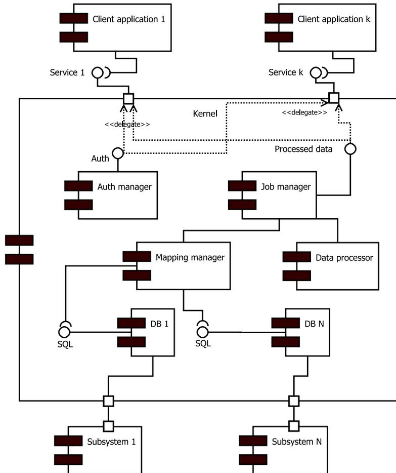
Figure 3.1: This UML component diagram provides a high-level software engineering schema of the city kernel: this module is designed to collect raw data from many different source, here called subsystems, and expose services for the urban context based on the processing of those data.
