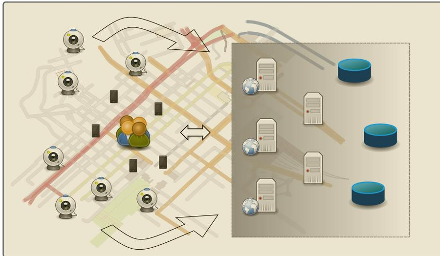
Figure 3.4: The WTC sensors scattered in the urban context constantly communicate the raw data about the urban traffic to the city kernel storage servers. The kernel's application servers expose a service that allows Android mobile clients to display real-time traffic information to the citizens.
