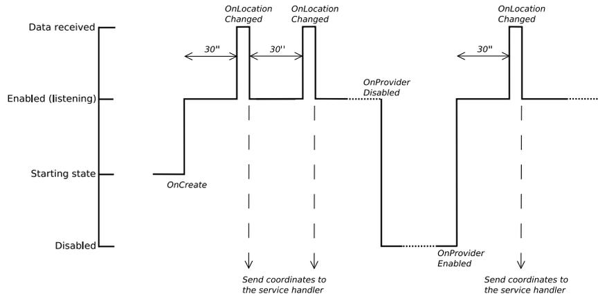
Figure 2.3: The timing logic behind the location thread; when gps or network listeners are enabled on the Android client the thread sends new coordinates to the Android application service every 30 seconds.
